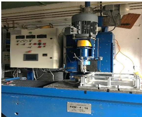
Figure 3 – FSP processing equipment [31]
