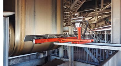
Figure 2 – Monitoring the state of steel wires [8]
